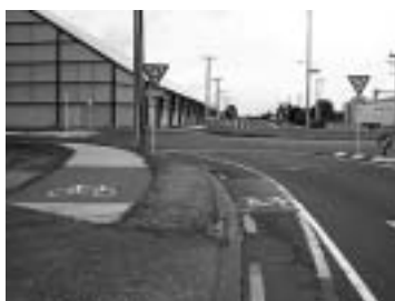
The experience levels of different types of users, particularly cyclists, may warrant redundant treatments such as these parallel on and off road cycle lanes and paths (Tauranga, New Zealand).
